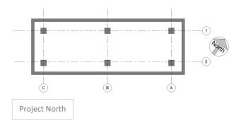
As standard a Project North will be set up. If a specific Project North is required, it would need to be specified before work commences.
