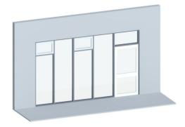
Curtain walls will be modelled to include accurate mullion positions and sizes. The location line will be placed so the glass sits in the correct position. Glass panels will be replaced accordingly by spandrel panels, doors or windows that accurately represent the feature of the curtain wall.
